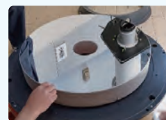
◀ The re-coated primary mirror of the 60 cm reflecting telescope
